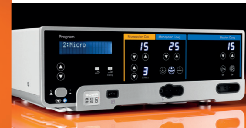
Finely regulated currents can be employed for the use of micro-needles in the Micro program
