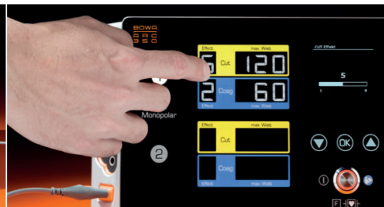
Simple to use: Tap the corresponding field to activate the input menu in the centre of the ARC 350 to adjust effects or power values
