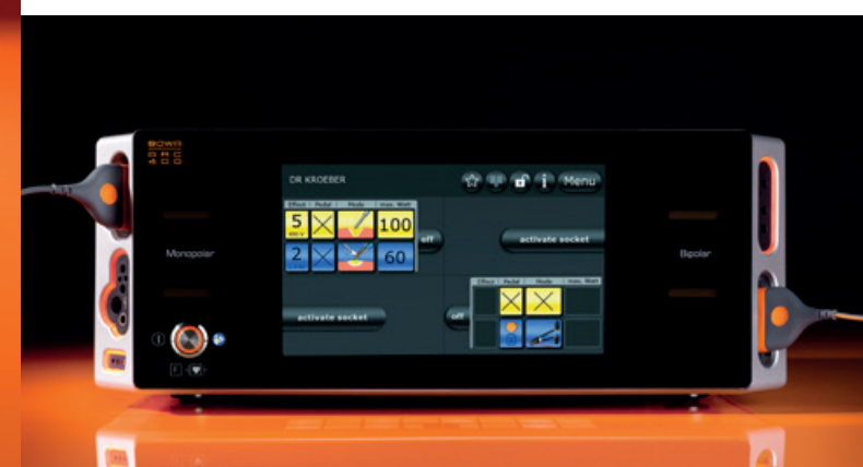
Clarity: Every connected socket – in this photo the upper left and lower right – is clearly assigned to one quadrant of the display
