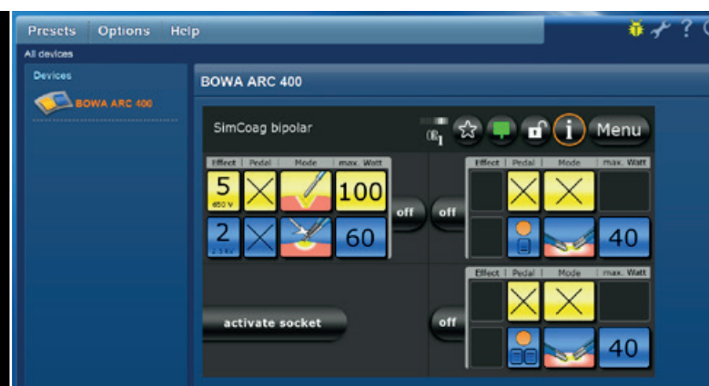
Professionals working together: Set the power, type of current and the activation type through the KARL STORZ OR1™
