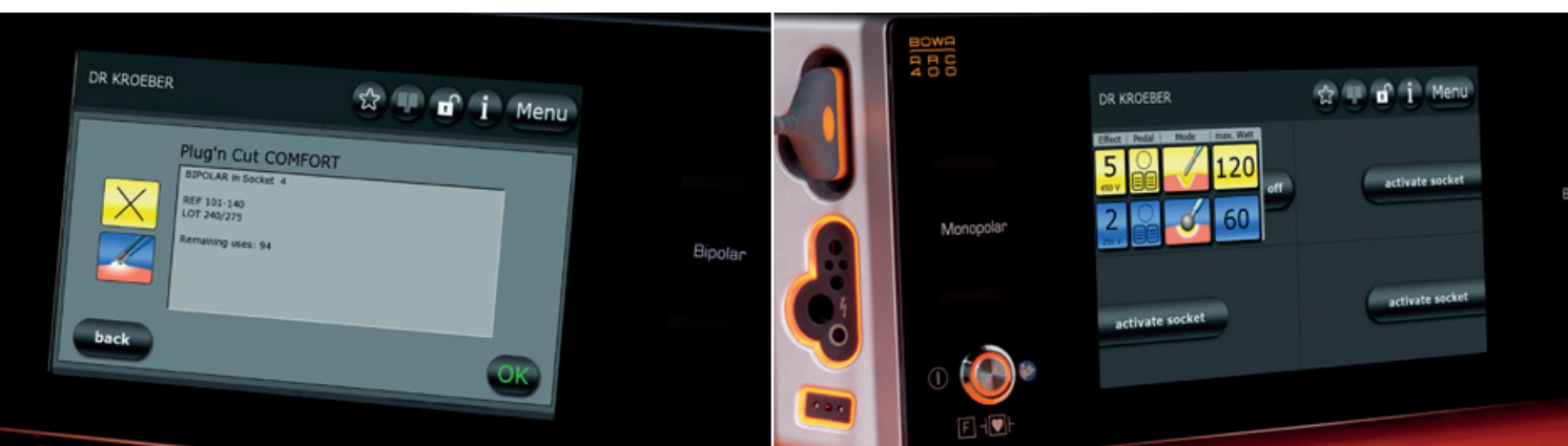
Plug'n Cut COMFORT: The COMFORT SYSTEM automatically recognises the COMFORT instrument, indicates how many times it may still be used and selects the correct parameters for the procedure
